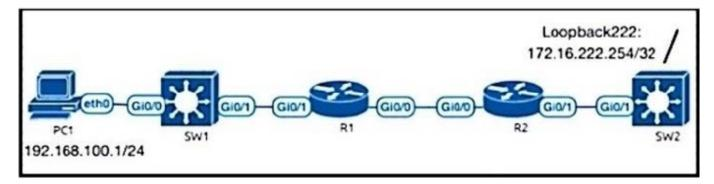
R2 can reach Loopback222, but R1, SW1, and PC1 cannot communicate with 172.16.222.254. R1 and R2 configurations are shown here:
