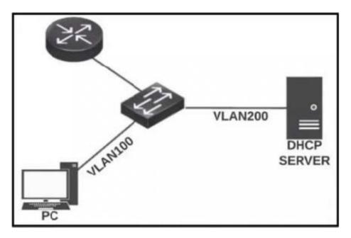
A PC is configured to obtain an IP address automatically, but it receives an IP address only from the 169.254.0.0 subnet. The DHCP server logs contained no DHCPDISCOVER message from the MAC address of the PC. Which action resolves the issue?
